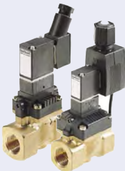
Type 6212 2/2 way, Servo Assist Solenoid Valves With Separating Diaphragm Isolating Media From Solenoid System. Option with Integrated Flow Switch for Brass Body Normally closed or normally open function
