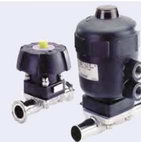
Type 2031 Pneumatic Operated Type 3233 Handwheel Operated Stainless Steel, 2/2 way, Diaphragm Valve Orifice size : 4.0 to 100.0 mm Kv : 1.0 to 235.0 m 3 /h Port conn. : Weld ends to DIN, BS, ISO, SMS Tri-Clamp to DIN, ISO, SMS, ASME (Other connections on request)
