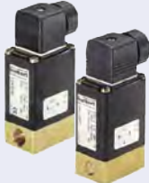
Type 0330 Type 0331 2/2 way, 3/2 way, Direct Acting Solenoid Valves With Separating Diaphragm Isolating Media From Solenoid System and with Manual Override Standard Normally closed, normally open, diverting, mixing or universal function
